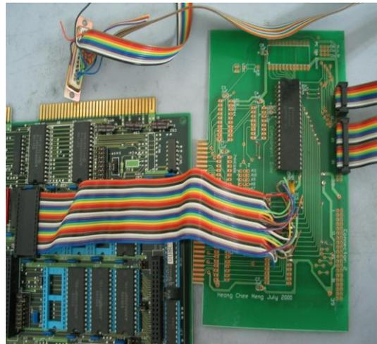
**Figure 2: Left: target system (Equipment embedded controller). Right: RAM emulator prototype uses an Intel 8255 PPA (digital IO) IC for communications with a Linux PC's parallel port.**
