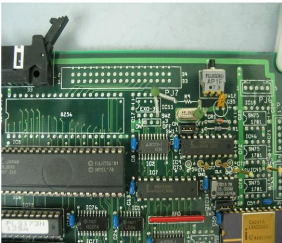
**Figure 7: Entry point via MB8256 UART IC. In many ways the ideal entry point. This is the original developer's IO port. Replacing all 5 ICs results in a working serial channel.**
