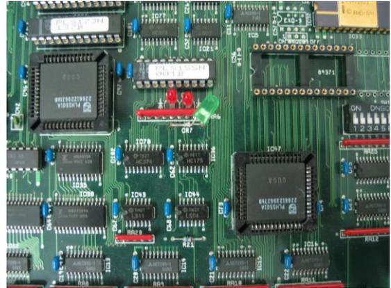
**Figure 8: Square ICs are PLDs implementing custom memory controller logic. This has to be probed. Top right: note only a portion of the MB89371 socket is used.**
