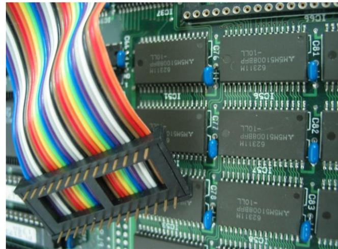
**Figure 4: Mechanical incompatibility between DIP-28 probe and SMD RAM packages in the controller**
